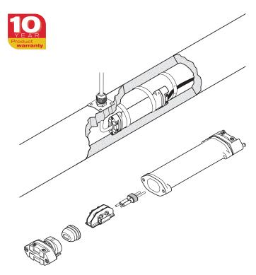
The nVent RAYCHEM C-150-E is a cold applied low profile power connection. The kit enables in line connection of nVent RAYCHEM industrial heating cables, BTV, QTVR, XTV and KTV, to a flexible power cable. It can be used in applications with temperature ratings from  $-55^{\circ}$ C to 200°C. It is approved for use in hazardous areas.
