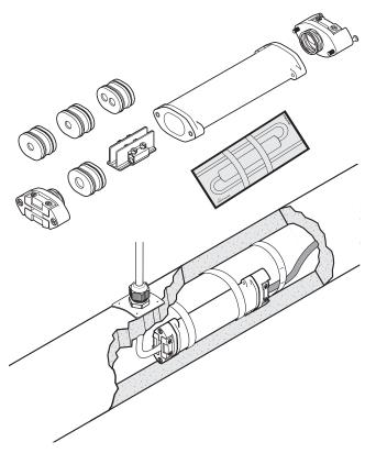
The nVent RAYCHEM CS-150-UNI-PI is a universal low profile heating cable connector for the direct connection of single conductor Polymer Insulated (PI) series heating cables. It can be used in different configurations: for the connection of a cold lead to a heating cable (Variant C), as an under insulation connecting system for the connection of a three core power cable to a heating cable loop (Variant L), as well as for splicing two heating cables (Variant S).
