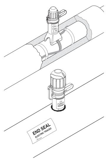
Both the nVent RAYCHEM E-100-E and E-100-L-E are accessible, re-entrable end seals, the E-100-E without a light, the E-100-L-E with a signal light. Both end seals can be used with all nVent RAYCHEM BTV, QTVR, XTV, KTV, HTV or VPL industrial parallel heating cables. They are approved for use in hazardous areas. They are extremely rugged - made of a strong, moulded part with 4 mm wall thickness.
