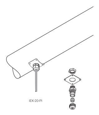
Insulation entry kits are designed to protect cables when passing through the thermal insulation cladding. The nVent RAYCHEM IEK-20-PI is suited for PI heating cables as well as for power cables.
