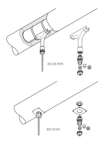
Insulation entry kits are designed to protect cables when passing through the thermal insulation cladding. The IEK's are suitable for all type of parallel heating cables as well as power cables. Insulation entry kits may be used in hazardous and non hazardous areas.
