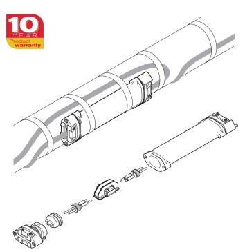
The nVent RAYCHEM S-150 is a cold applied low profile splice for in-line connection. This universal kit fits with all nVent RAYCHEM industrial heating cables, BTV, QTVR, XTV and KTV, meaning simplified product selection and reduced inventory to stock. It can be used in applications with temperatures ranging from -55°C to 200°C. It is approved for use in hazardous areas.
