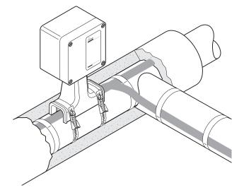
The nVent RAYCHEM T-100 is an above-insulation splice or tee kit, designed for use with up to three nVent RAYCHEM BTV, QTVR, XTV, KTV, HTV or VPL industrial parallel heating cables. It is approved for use in hazardous locations.
