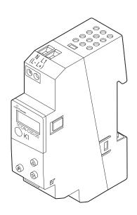
The nVent RAYCHEM TCON-CSD/20 is a compact digital thermostat for simple ON/OFF temperature control. The temperature is measured through a temperature sensor and shown on a LCD display. The actual status of the output relay is signaled via a LED.
