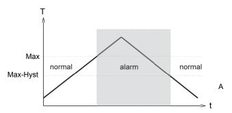
switchover delay time  $(t_{\text{DS}})$  can be applied to the switchover to the alarm state. Equally, one switch-back delay time  $(t_{\text{DR}})$  of several can be applied to switching back to the normal state.
