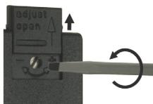
Turn clockwise for a lower switching point; turn anticlockwise for a higher switching point.
