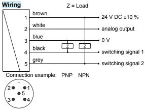
Before the electrical installation, it must be ensured that the supply voltage corresponds to the data sheet. The use of shielded cabling is recommended. Dimensions
