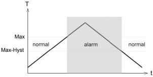
While in the normal state the switching outputs are at the level of the supply voltage; in the alarm state they are at 0 V, so that a wire break would also display as an alarm state at the signal receiver.
