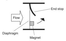
There is a plastic-coated magnet on the diaphragm. When there is a deflection, its magnetic field changes, and this is detected by a sensor outside the area of flow.
