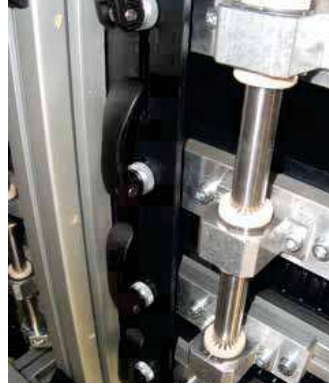
otion line should be adjusted without setup time ired. drylin® linear guides, which enable precise djustment, were used for this.
