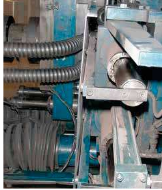
ng over to the drylin® R linear plain bearing, the ce rate of this compaction unit could be extended ars, despite high stressing from powder particles ive agents.
