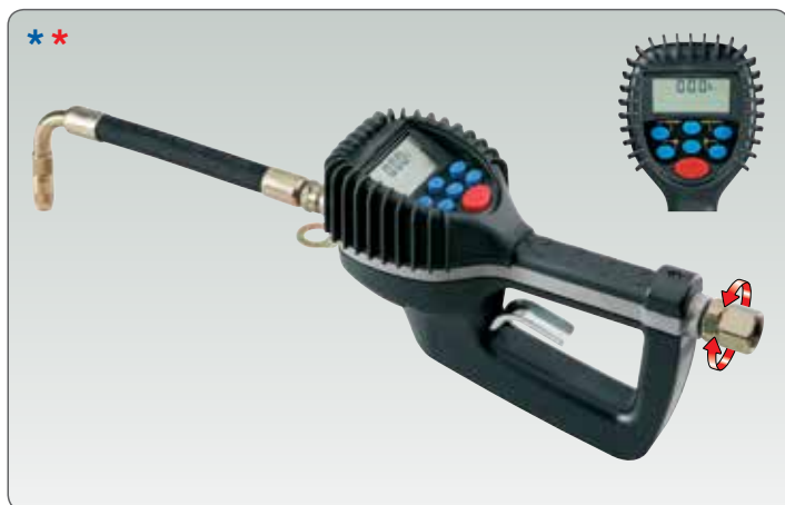
Art. 37704 Digital dispensing oil gun with preselection, equipped with: - inlet swivel joint F 1/2" - flexible terminal - semiautomatic nozzle ø 16 mm
