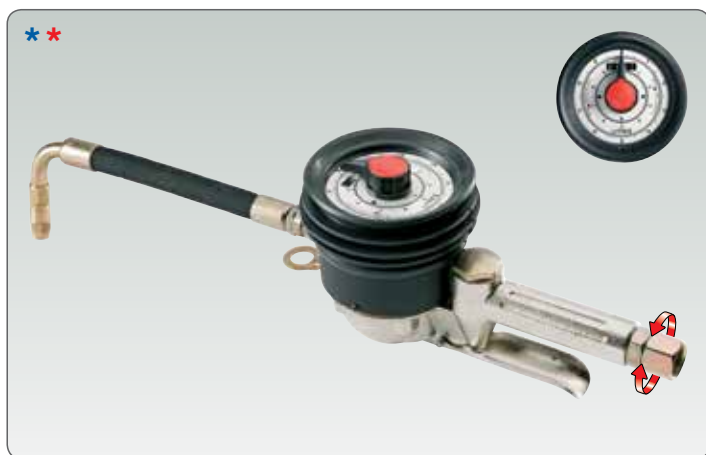
Art. 37703 Oil gun with mechanical litre-counter (Art. 37701), equipped with: - inlet swivel joint F 1/2" - flexible terminal - semiautomatic nozzle ø 16 mm
