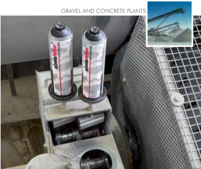
Two 250 ml simalube lubricators with brushes lubricate and clean the chain drive of a drum washing machine.
