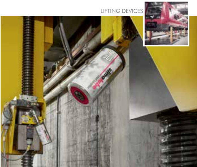
The spindles of a lifting station for railway wagons and locomotives are lubricated with 125 ml simalube over 12 months.
