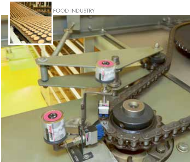
The drive chain of a transport belt, which allows rolls to cool, is cleaned with special blue brushes and lubricated with 2 simalube SL18 in 30 and 60 ml sizes.
