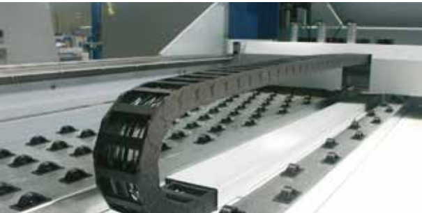
chainflex® CF130.UL for woodworking application. e-chain®: E4/light
