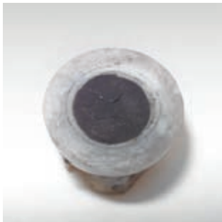
Clogged nozzle (back side)
