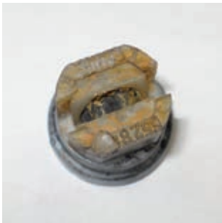
Clogged nozzle (front side)
