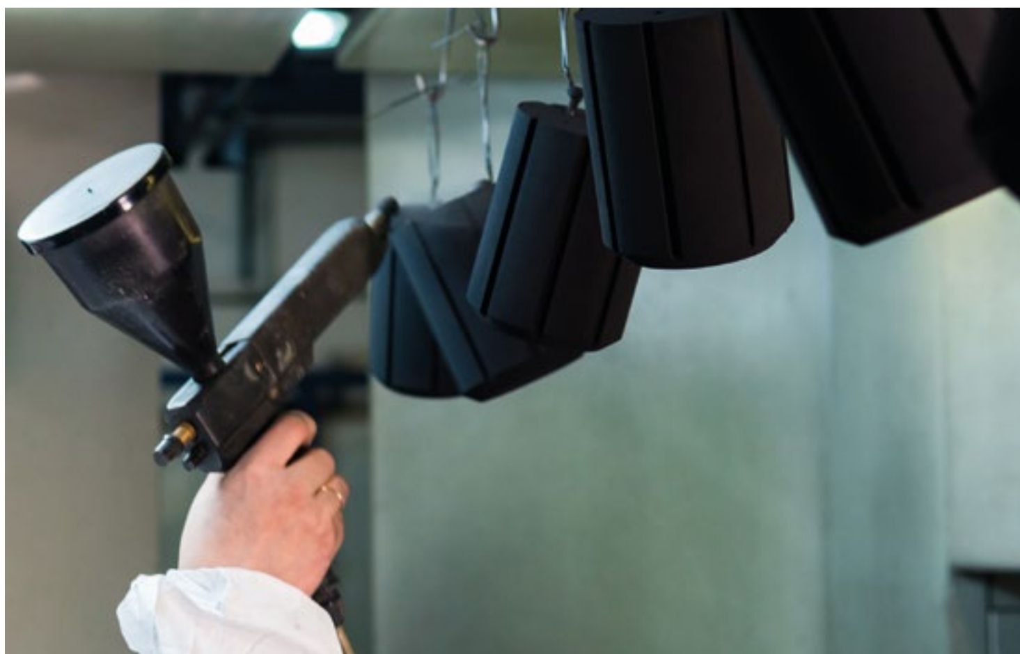
Powder coating of hanging components
