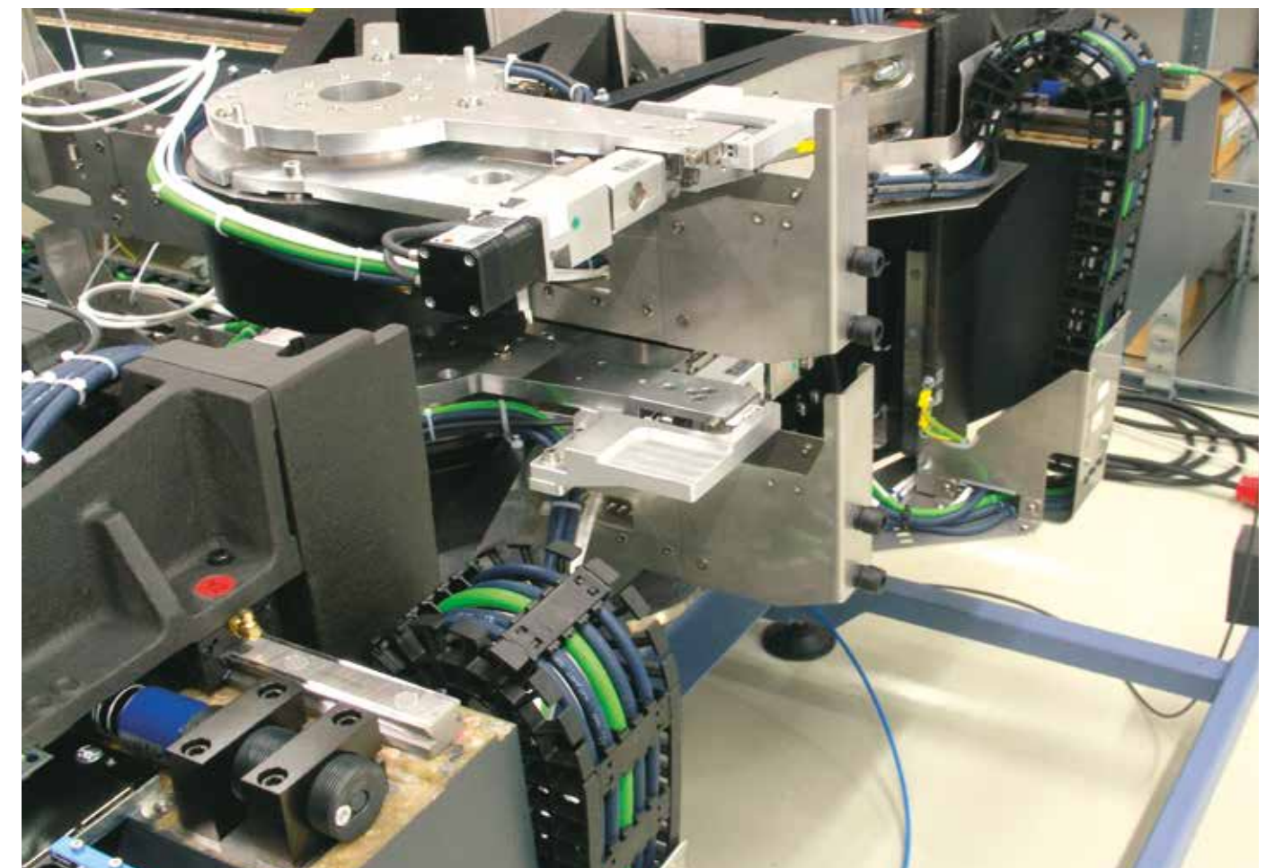
T3 system on the Z-axis of a positioning system. It has very low noise and vibration
