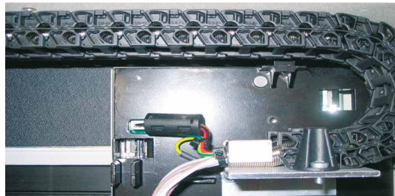
igus® E3 system, ideal for very small installation spaces as well as very low-noise operation
