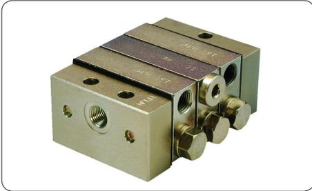
This group has only one outlet on each side of the section and is not equipped with built-in check valves.
