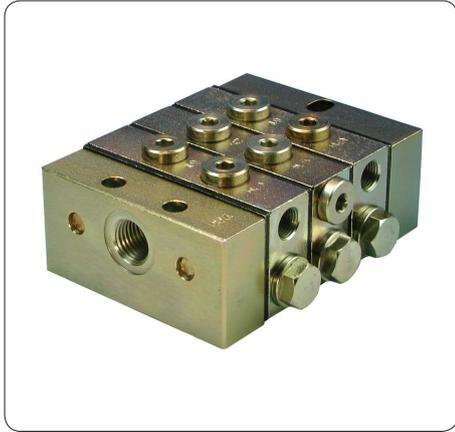
In this group, the feeder sections have two outlets on each side, one each on the side and one on top, but only one may be used. The second outlet must always be kept closed. These feeders are supplied with a built-in check valve.
