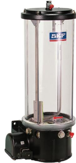
The pumps comprising the KFG group have 3 lubricant outlets for the connection of 3 progressive feeder circuits independent of each other. A separate pump element is required for each outlet port.
