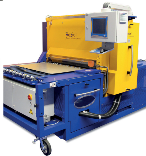
Blank lubricator system with 2 medium circuits
