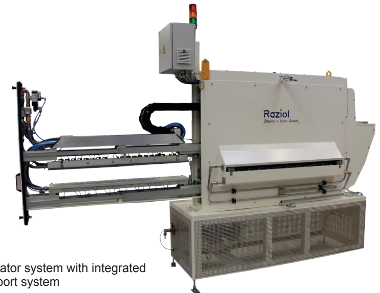
High-performance lubrication system for blanks, can be moved completely out of the line
