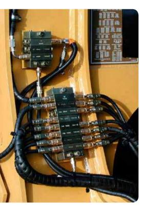
In progressive automatic lubrication systems, a piston pump supplies a defined amount of lubricant through the main line to the metering device that serves each outlet. SKF ProFlex and Lincoln Quicklub systems are designed for specific applications and can be configured to meet the unique lubrication requirements of every lubrication point on the equipment.
