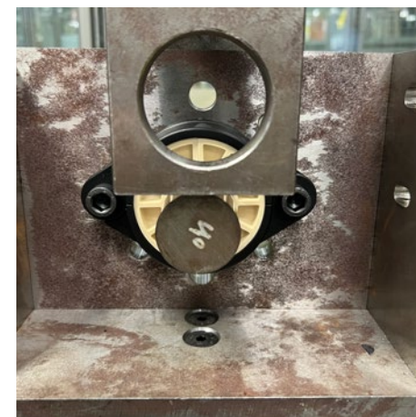
The split PTFE-free igubal® flange mounted bearing made of igumid® G and iglidur® J3 in compressive strength test.
