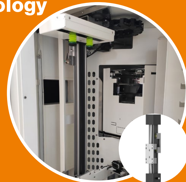
ZLW toothed belt axis moves the platform vertically
