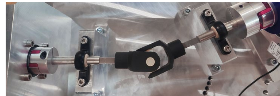
The UJM universal joint tested with 25° deflection.
