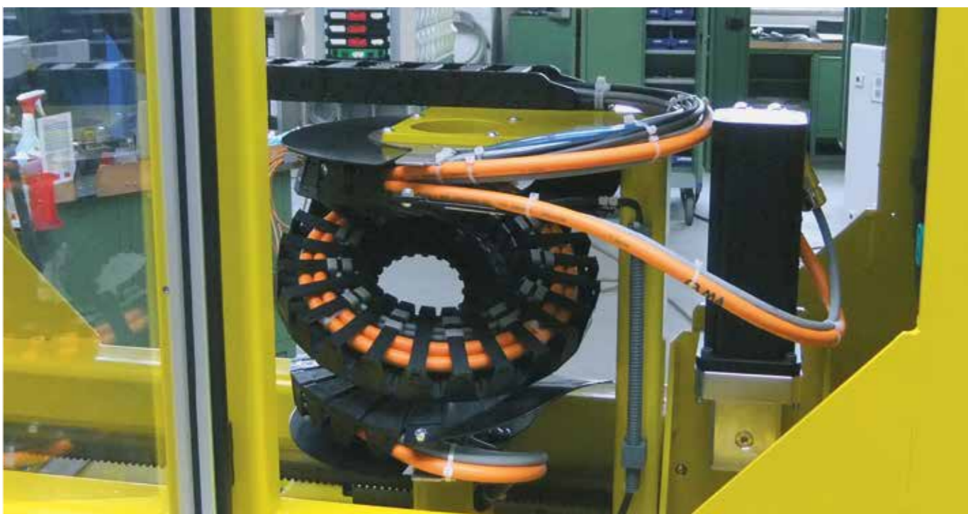
igus® twisterband TB30 for circular movements up to 360°, E2 mini and E2/000 e-chains® are used in this loading and unloading unit
