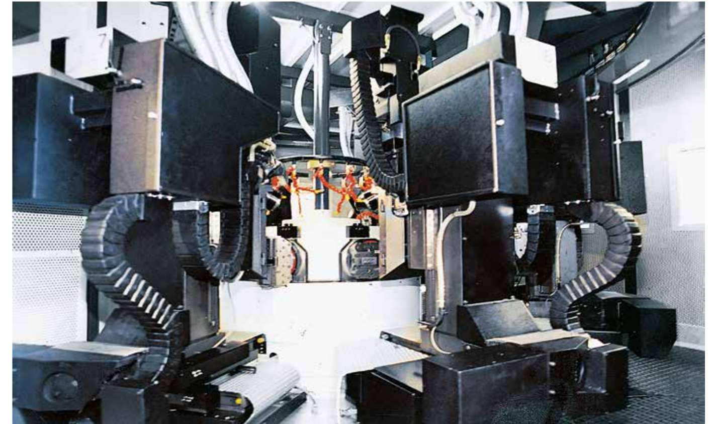
Various triflex® e-chains® on a machining centre
