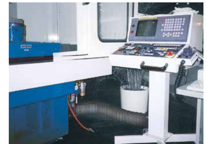
triflex® 332 as unsupported link from machines to control panel
