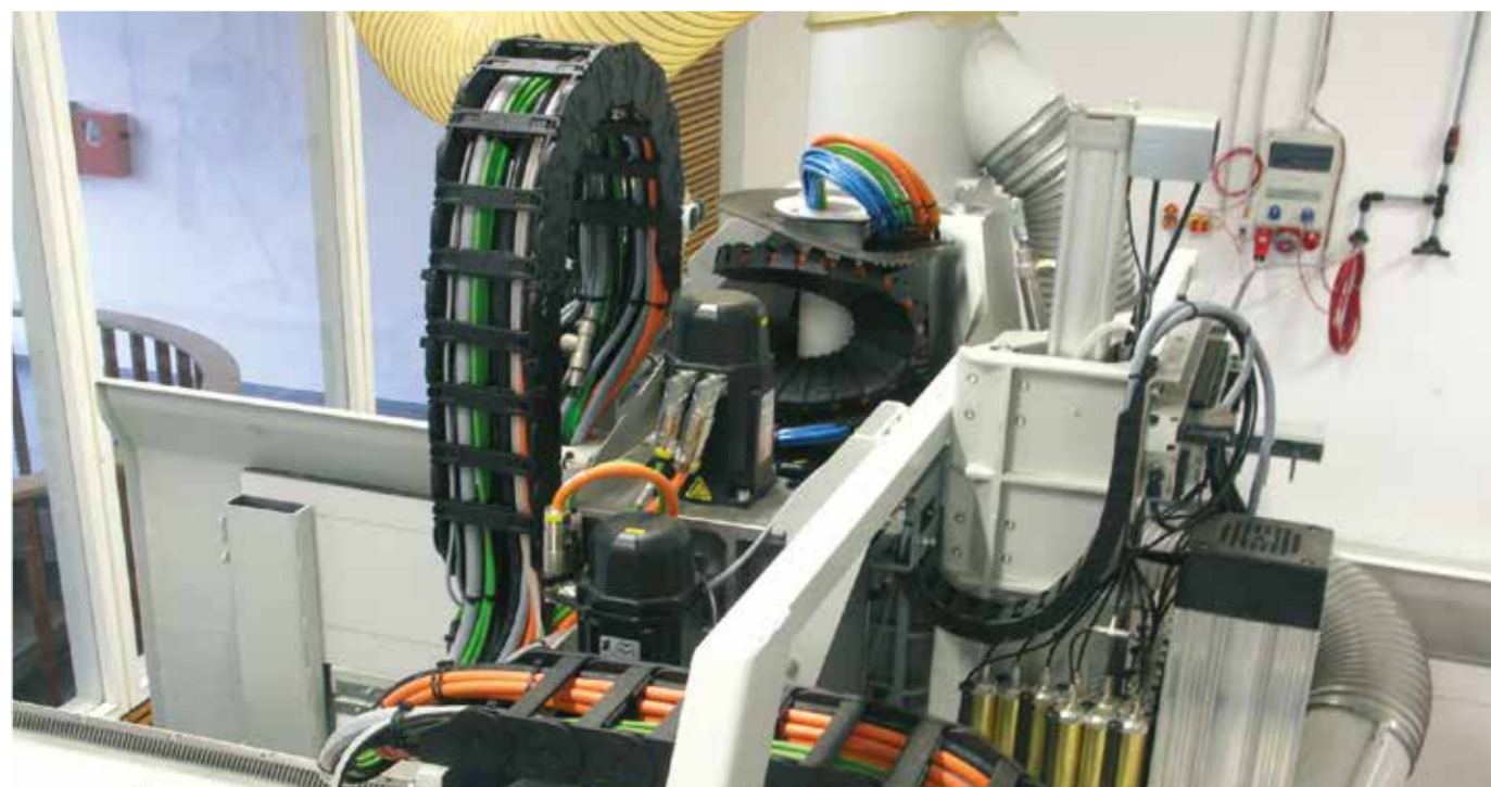
igus® twisterband and other e-chains® in a wood working machine
