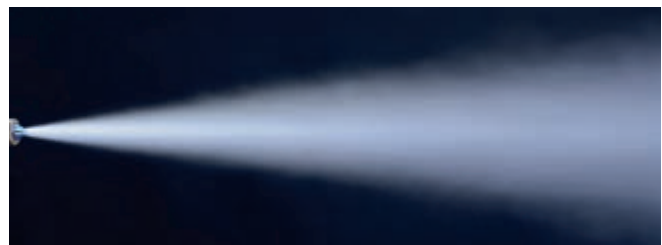
Spray pattern of a Laval nozzle
