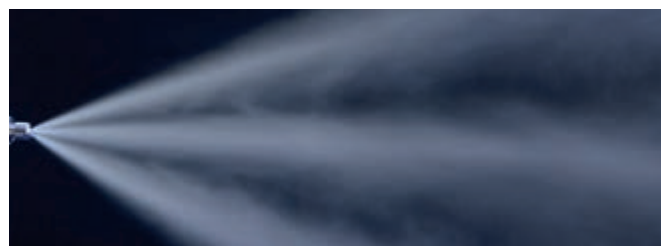
Spray pattern of a flat fan nozzle
