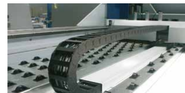
chainflex® CF130.UL for woodworking application. e-chain®: E4/light
