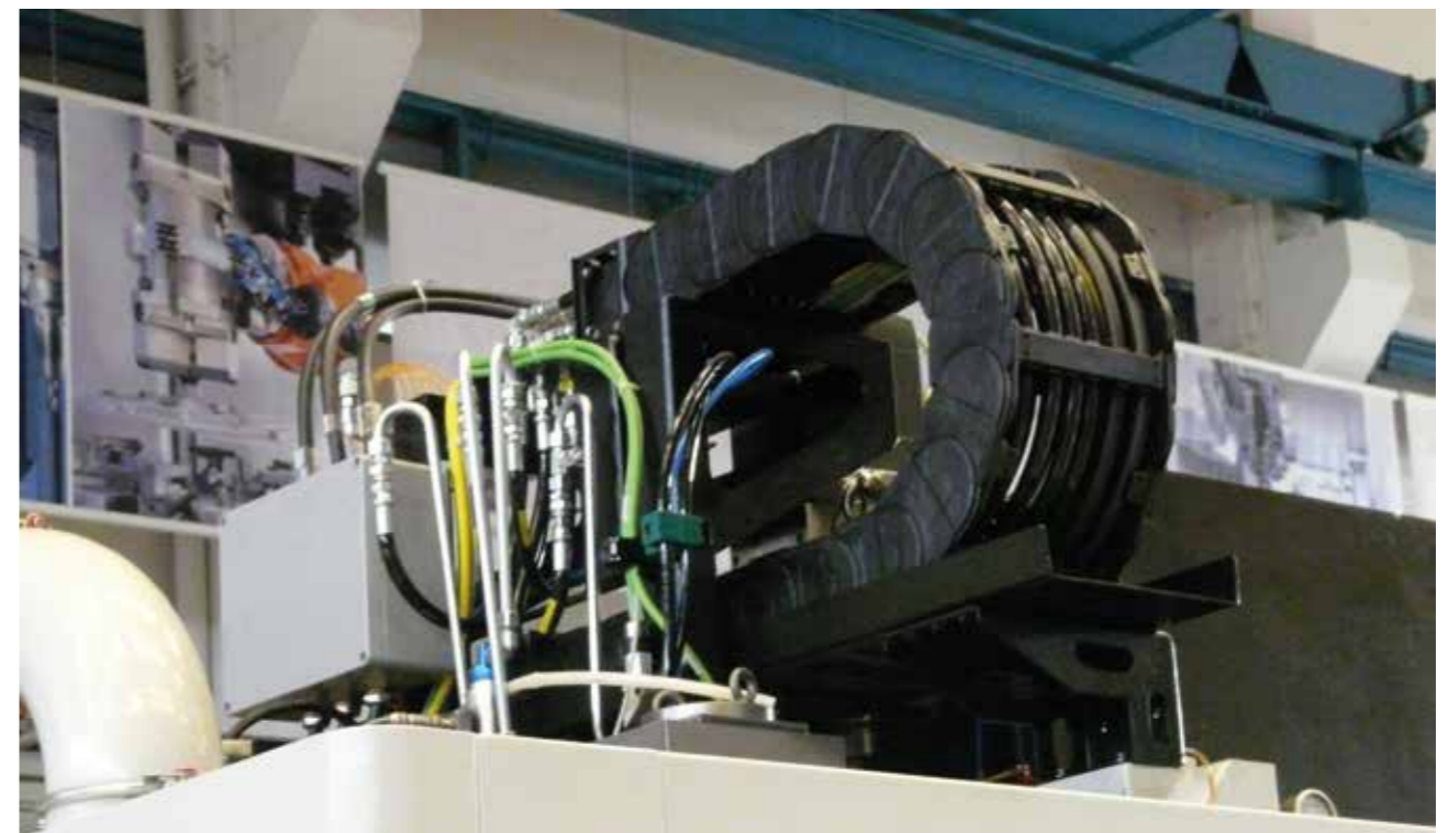
chainflex® CF880 in a short travel application
