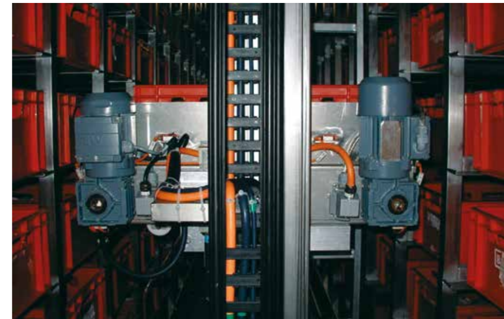
chainflex CF10 control cable in storage and retrieval units e-chain®: E2 system
