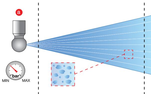
Figure 3: Rotating cleaning nozzles with recommended operating pressure
