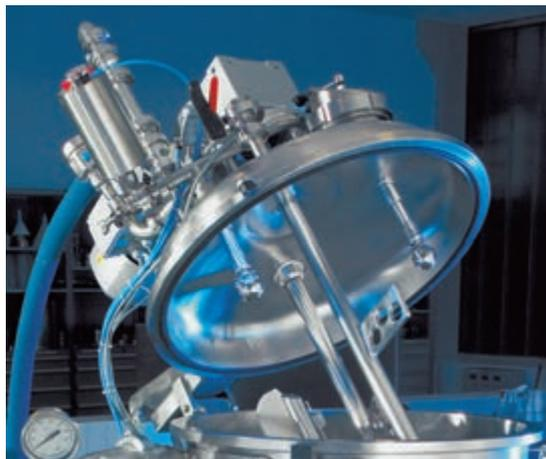
Many of Lechler's precision nozzles for tank and equipment cleaning are CIP-capable and can remain in the installation during the production process.
