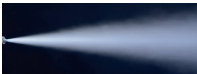
Spray pattern of a Laval nozzle
