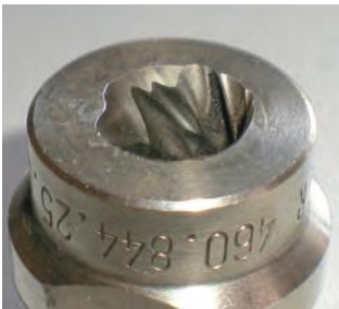
Fig. 2: Wear of a full cone nozzle
