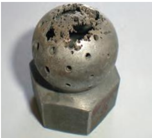
Fig. 1: Chemical corrosion of a spray ball
