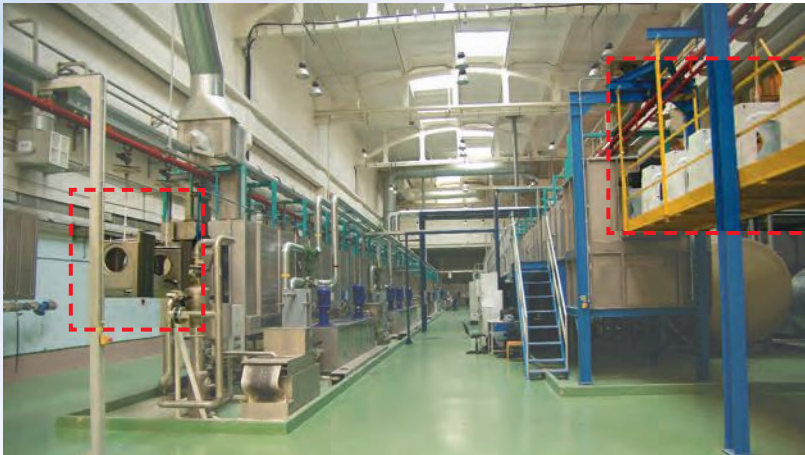
Example of a painting line for washing machine housings. On the left the component before painting, on the right the painting housing exits.
