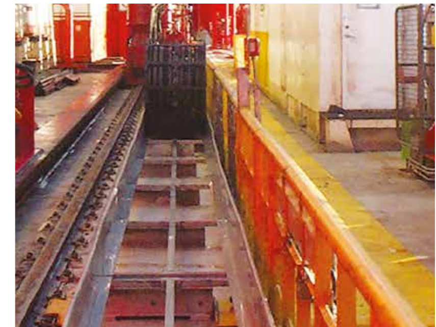
System E4 with extension links and high fill weight - long travel application on-board West Navigator drill ship
