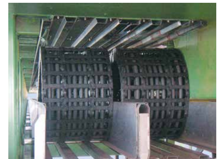
igus® system E4 with extension link on a ship loader for coal handling. Travel 105m, speed 240m/min, fill weight 53kg/m
