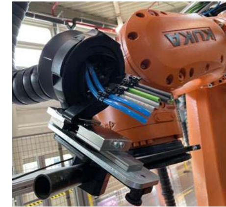
The sensor unit measures tensile forces using a 200kg load cell. It is assembled on the quick exchange kit for the axis 6 clamp.
