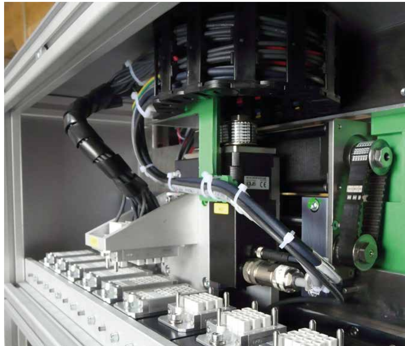
chainflex® CF31 motor cable in a fast picker
