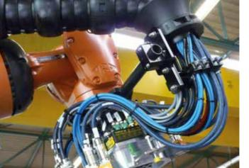
CFROBOT® cables used in robots for the automated systems in fuel tank production. These are supplied as fully harnessed readychain® systems.
