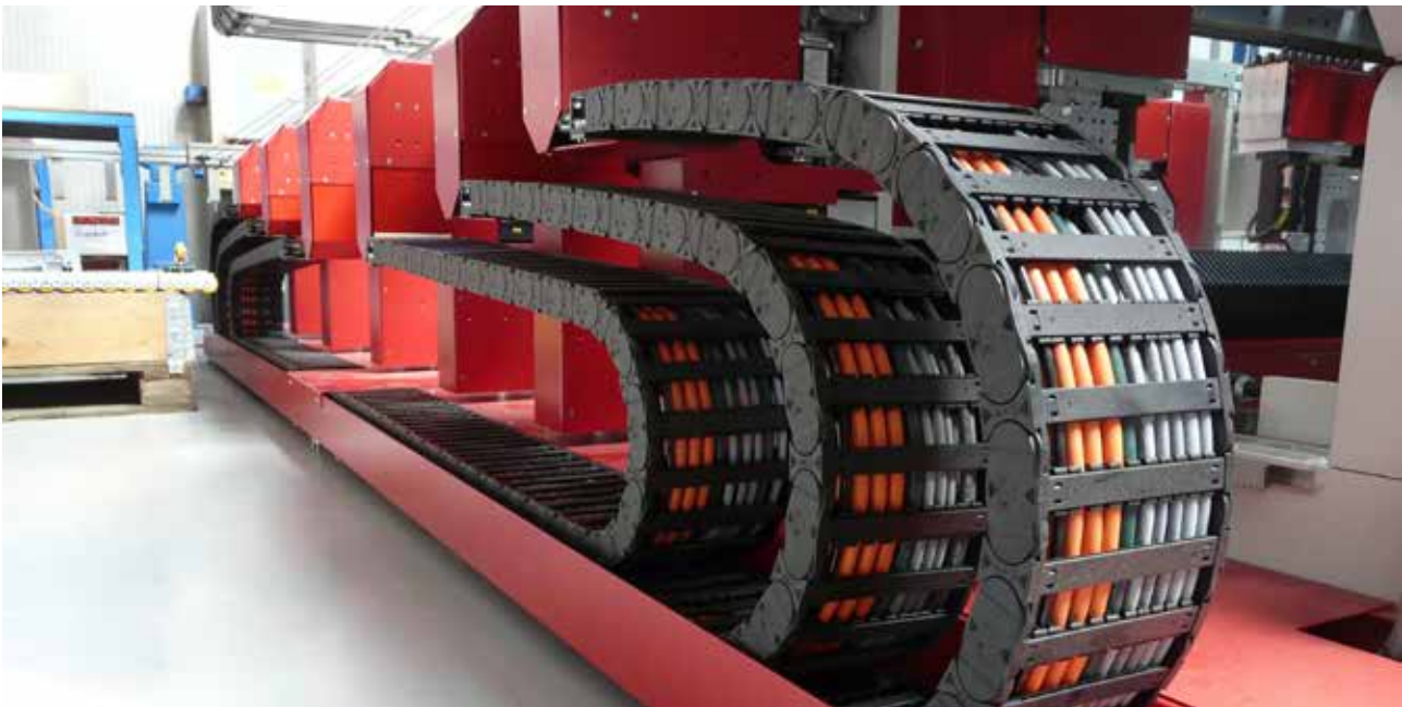
Drilling machine for wooden plates equipped with latest hybrid cable technology with Hiperface DSL
