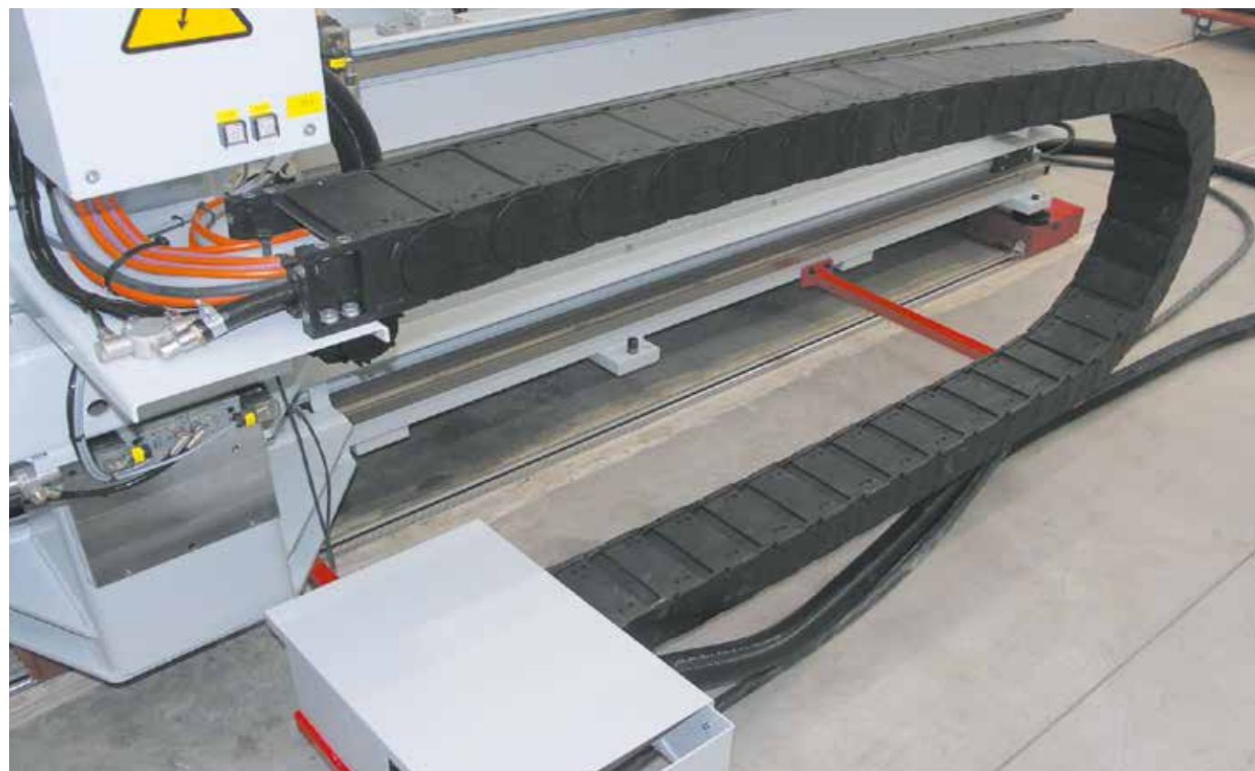
E4/light e-tubes protect cables and hoses against dirt and swarf
