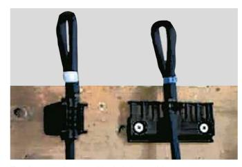
Tensile strength tests with chainflex® cables
