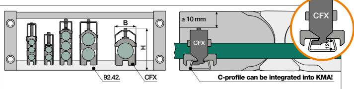
The H dimension in the tables is based on the maximum cable diameter. Cables with smaller diameters may result in a lower overall clamp housing heights. Tightening torque for CFX clamps 1.5Nm.
