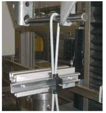
igus® tensile strength test CFX clamps with stacker saddle. Conclusion: the tensile strength of igus® chainfix clamps is three times higher when compared with conventional strain relief
