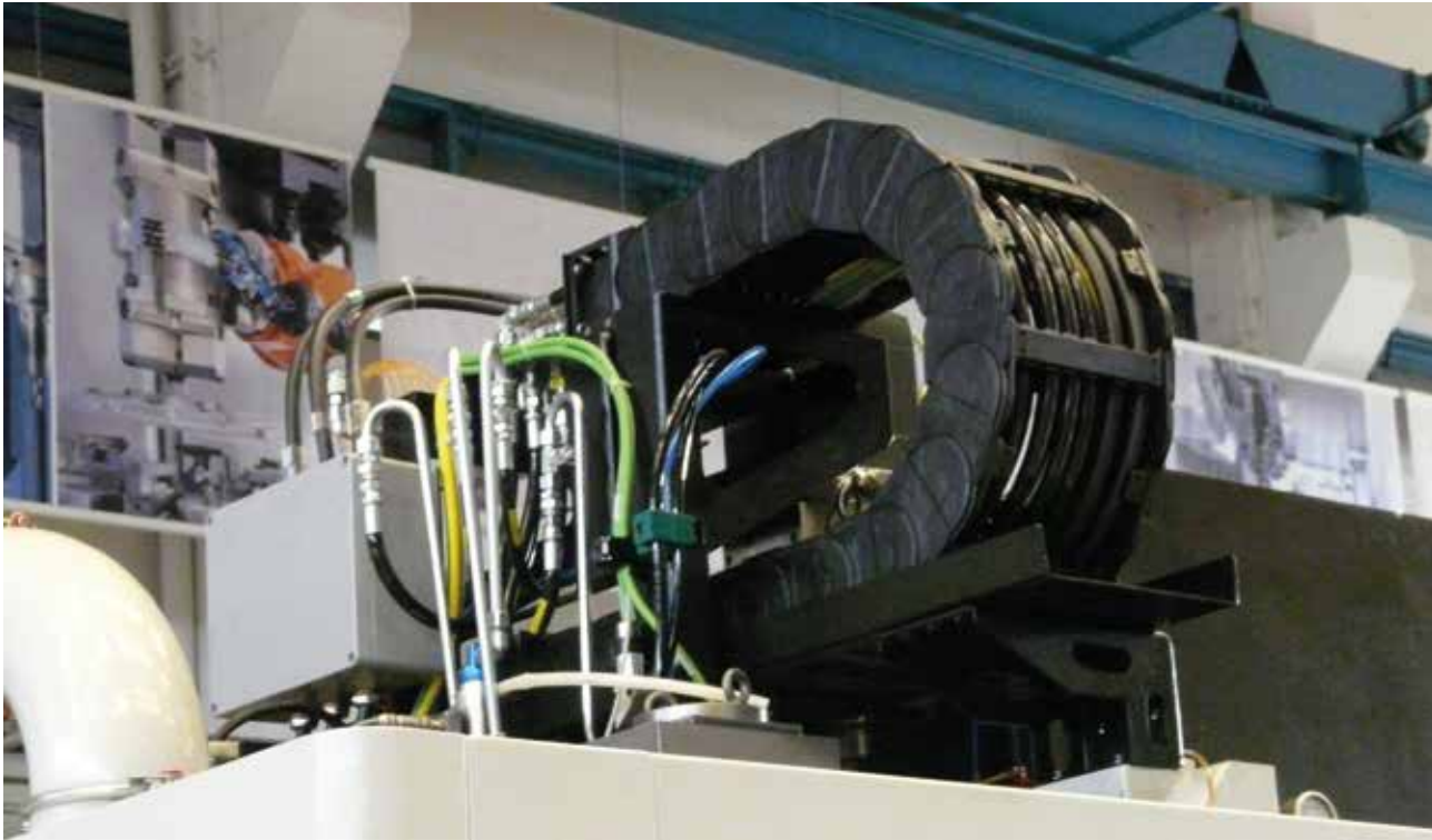
chainflex® CF880 in a short travel application
