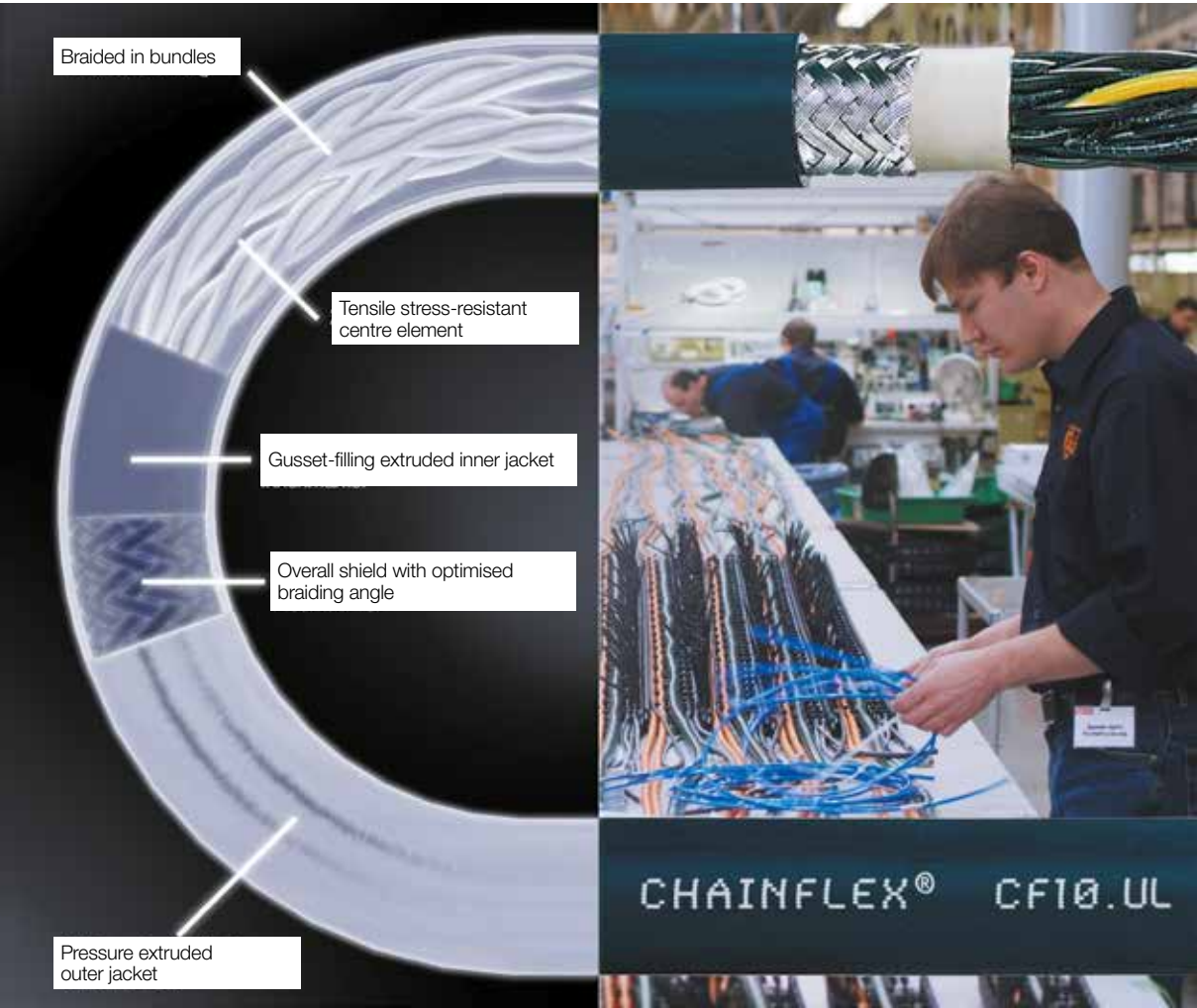
The special cable structure of chainflex® CF10.UL guarantees quality – offered by igus® fully harnessed.
