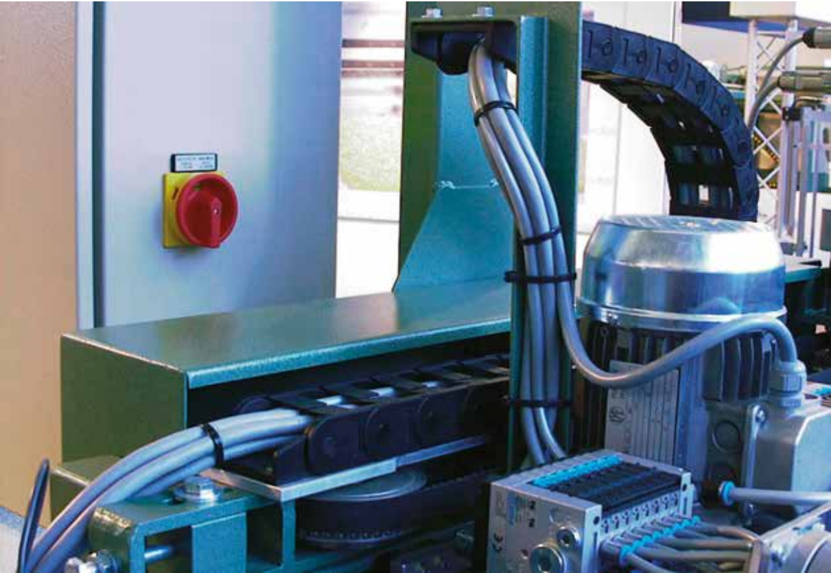
chainflex® CF140.UL in a feeder application. e-chain®: easychain®
